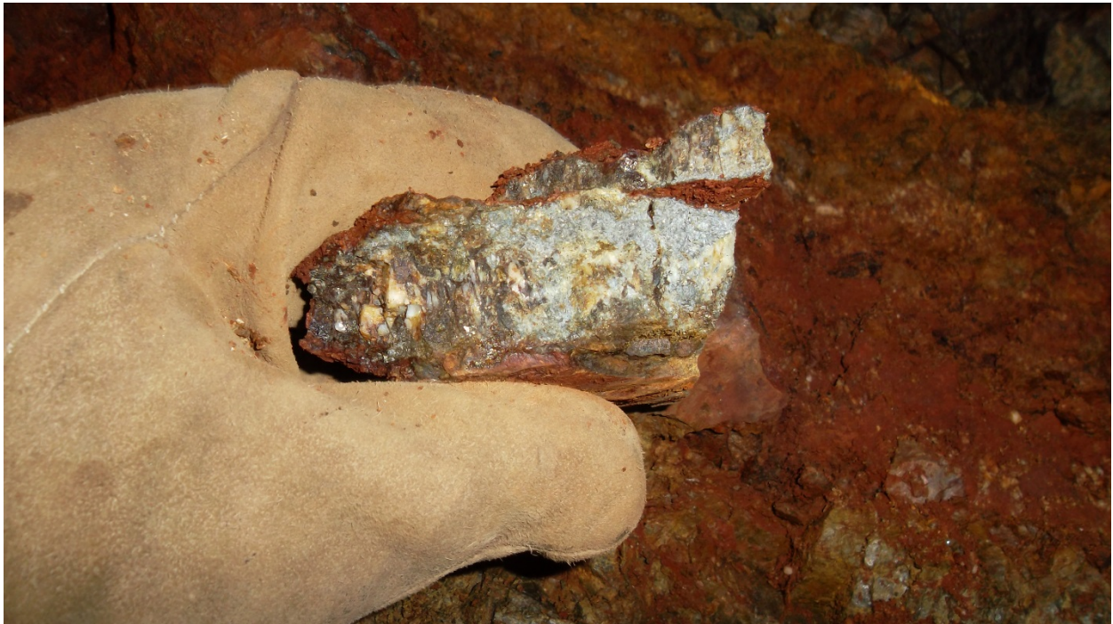
Vein 1 , Arsenopyrite vein w/quartz. .16opt, 2 opt silver, .15% cu, 234 ppm bismuth
